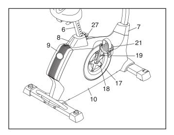
Next, remove the Adjustment Knob (27) and remove the Seat Post (6).
