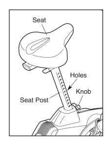
in one of the adjustment holes in the seat post. Then, tighten the knob.
