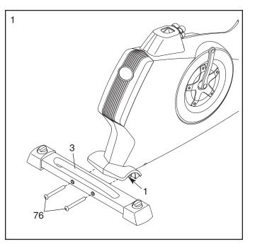
2. Attach the Front Stabilizer (2) to the Frame (1) with two M10 x 95mm Patch Screws (76).
