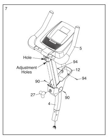
8. Slide the Front Shield Cover (7) upward onto the Upright (4).
