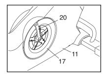
Rotate the left Pedal Disc (17) clockwise to release it from the Left Shield (11). Then, work the left Pedal Disc upward and remove it from the Left Crank Arm (20).
