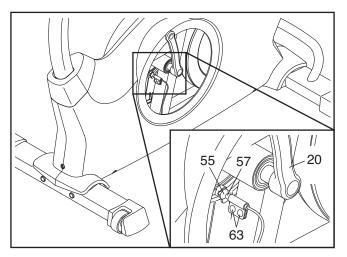
Next, rotate the Left Crank Arm (20) until a Magnet (55) is aligned with the Reed Switch (57). Slide the Reed Switch slightly toward or away from the Magnet. Then, retighten the M4 x 12.7mm Flange Screws (63).
