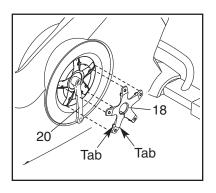
Using a flat screwdriver, release the tabs on each point of the left Disc Cover (18). Carefully work the left Disc Cover over the Left Crank Arm (20) and remove the left Disc Cover. Next, rotate the Left Crank Arm (20) to a vertical position with the end of the Left Crank Arm pointing upward.
