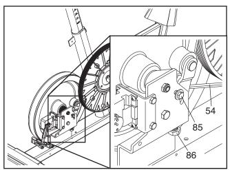
When the Drive Belt (54) is tight, tighten the M6 x 20mm Hex Screw (85).
