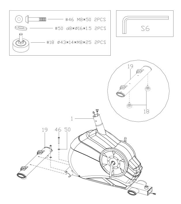
**STEP 2** Thread Foot Pads (18) on the Main Frame (1).
