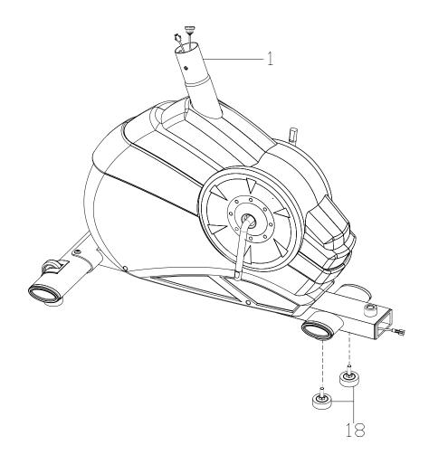
Thread Foot Pads (18) on the back Bottom Tube (30).
